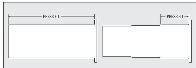
**CAUTION:** When step machining the bearing shell material, do not reduce the original shell material wall thickness by more than 50%
